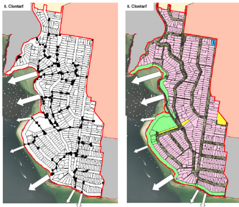
Figure 3E: Clontarf Catchment. (Left) artificial stormwater drainage network. Arrows indicate stormwater outfall locations (Right) land-use breakdown (Pink: residential; Green: open space; Clear: roads; Blue: commercial; Yellow: special use).
