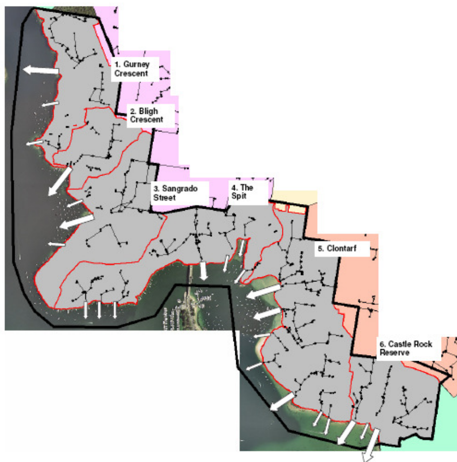
Figure 2: The six Clontarf / Bantry Bay Catchments in Manly Council (shaded grey with red boundaries). Top-to-bottom: 1. Gurney Crescent; 2. Bligh Crescent; 3. Sangrado Street; 4. The Spit; 5. Clontarf; 6. Castle Rock Reserve. Artificial stormwater drainage networks are shown by black lines within the catchments. Black dots indicate locations of pits. Arrows indicate stormwater outfall locations; major outfalls are indicated by larger arrows. The Spit Bridge is visible on the centre-bottom.
