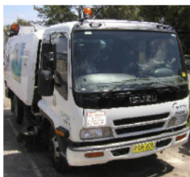
Figure 6: Schematic of a typical Schwartz regenerative air street sweeping vehicle used in the Manly LGA.
